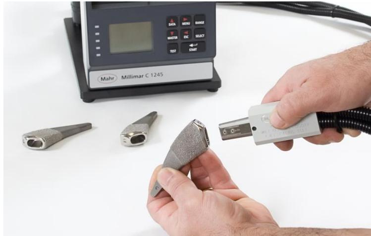
*-- Multiple jetting and spacers allow one tool to be used on many tapers, regardless of length*
